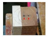
Start by marking the centre of the blank (Centre A) and then make another mark at about 15 mm away from point A, (centre B).
