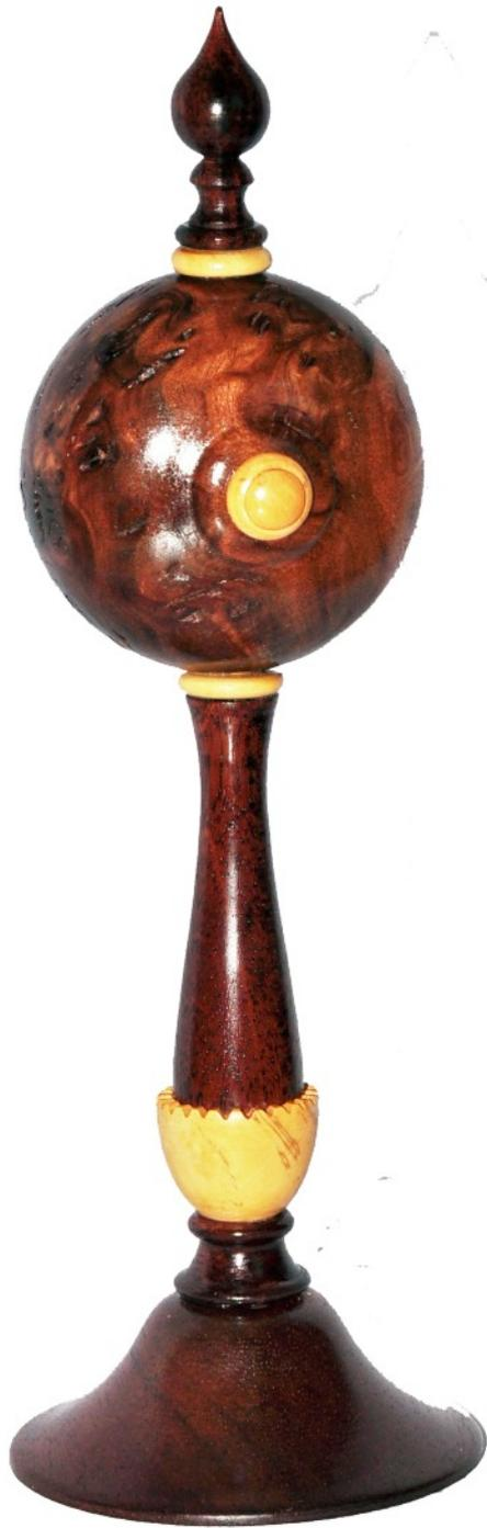
The 24 serrations in the boxwood are effected by a triangular file as shown in the article. Using the index system of the lathe to mark the position of each serration is one option. Another option is to use a template which is cut out and stuck to the top of the boxwood. Mark each line carefully with a stanley knife and then file each nick.
