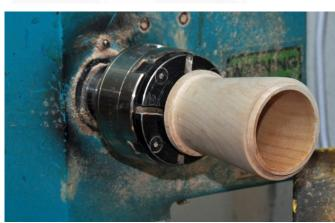
Before hollowing commences drill a 13 mm diameter hole in the centre to the required depth. A 10 mm gouge fits into this hole and facilitates bevel-rubbing as you start hollowing outwards from the centre alternatively something like the Sorby midi multi purpose hollowing tool might be preferred as it is forgiving and nice to use. A scraper can be used to refine the end grain. Lightly shear scraping the final cuts can usefully reduce the amount of sanding required.
