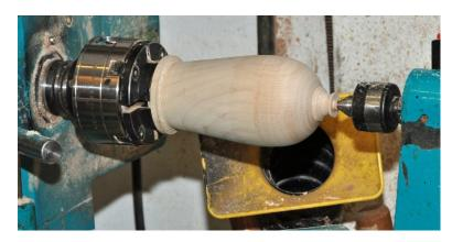
Before shaping the outside of the lid I fit the lid to the base because it is then easier to achieve a continuous curve.
