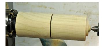
Part off about half the cylinder and put to one side. This will be used to make the lid with finial.
