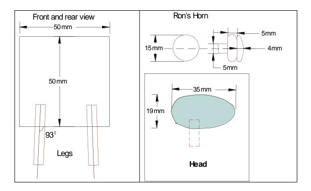
Having drilled holes for the legs a hole is required to take the dowel to fix the head and another hole is required to fix the tail. I turned my own pins but using 6mm dowel sold in lengths by hardware stores is quicker and convenient.
