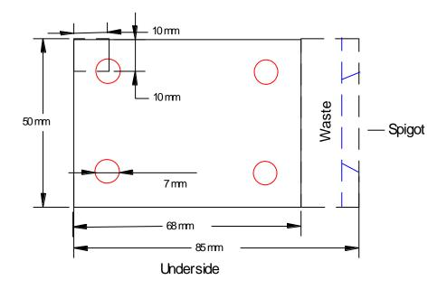
You may find it easier to drill the holes in the body for the legs, head and tail while it is in square section. The leg holes are positioned 10mm from the front and back edge using a 7mm thick drill bit. The drawing below shows that the legs are drilled at a slight angle.
