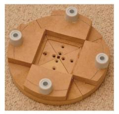
The MDF pieces mounted on the main body allow me to grip square section of 90mm and above
