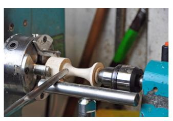
8. Finish shaping with ¼ inch spindle gouge. Sand and apply a finish then part off . Glue roof to body and fit perch.
