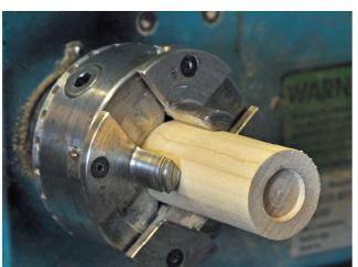
4. Shape the bird box with a spindle gouge . For the finer detail a ¼ inch spindle gouge is my tool of choice.
