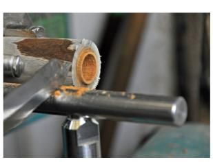
3. With a parting tool make a 2 mm rim on which to locate the roof .
