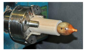
6. Before shaping the roof check that the body fits snugly in this recess.
