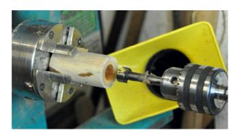
2. Mount the blank between centres and turn down to a cylinder.
