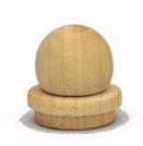
Sand and finish. Avoid finishes that have toxic chemicals. Boiled linseed oil and pure beeswax can be used successfully as here although any food safe finish could be used.
