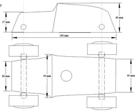
Now blend the bonnet with the rest of the car moving the timber between Centre A and B as necessary. Remove the work from the lathe and saw the wood lengthways so that the car has a flat bottom and a small flat area on the top surface of the car.
