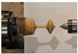
4. With most of the heavy cuts out of the way the tailstock can be removed completely. Finish the stem with the side of a gouge to produce a slight taper. Sand, decorate and finish with sander sealer or oil and part off. Now for the moment of truth will it spin?
