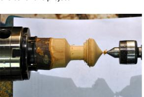
**3.** When you are happy with the pointy end of the top reduce the width of the cylinder with a parting tool as shown. Give yourself some access space by turning away some of the waste wood.
