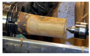
**1.** Mount the wood firmly in the chuck, bring up tailstock and turn down to a cylinder with the roughing out gouge. I find fruit wood is a good choice for this project.
