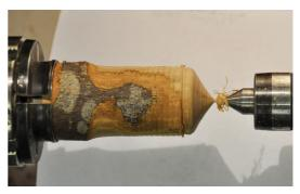
2. Shape the end to a point (not too fine a point or it will break) with a 3/8ths spindle gouge. The tailstock is not in contact with the wood but close enough to limit the wood making its own way in the world.
