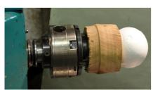
When the ball fits snugly inside the bowl bring up the tailstock. Take only light cuts to the foot of the bowl
