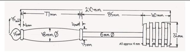
**Stage 2:** Move on the handle end which should be at the headstock of the lathe. Shaping can be done initially with the SRG (spindle roughing gauge) and finally with the skew or spindle gauge.
