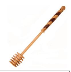
Foreword: The dipper can be made in sections if turning such a long thin stemmed piece is a worry. However by supporting with fingers and using a skew to plane down the stem, it can be achieved from one piece.
