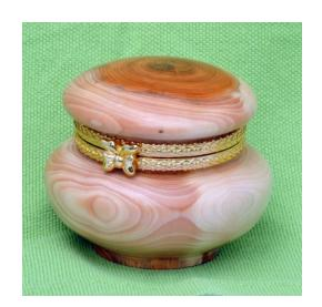
This hinged box is a relatively straightforward project. Start with some pretty wood (yew is ideal) about 80 mm wide and 80 mm long. Mount the wood between centres and rough to a cylinder forming spigots at both end. Part off about a third of the cylinder and put to one side. This will be used to make the top of the box.
