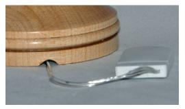
This hole with the recess provides an exit for the wire and switch/battery housing
